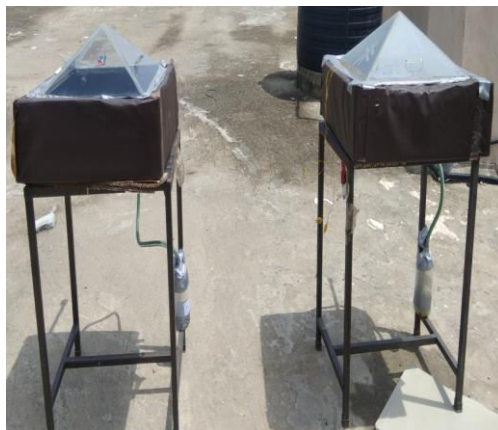
Fig. 3. Schematic of distillation still and distillation of waste water after filtration
