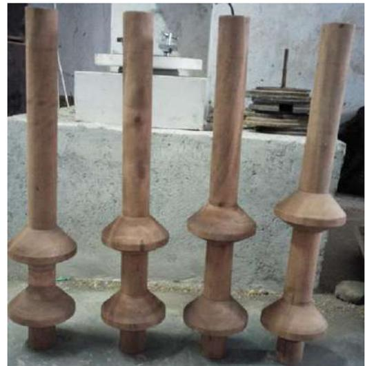
**Fig. 2.** Models of double under-reamed piles.
