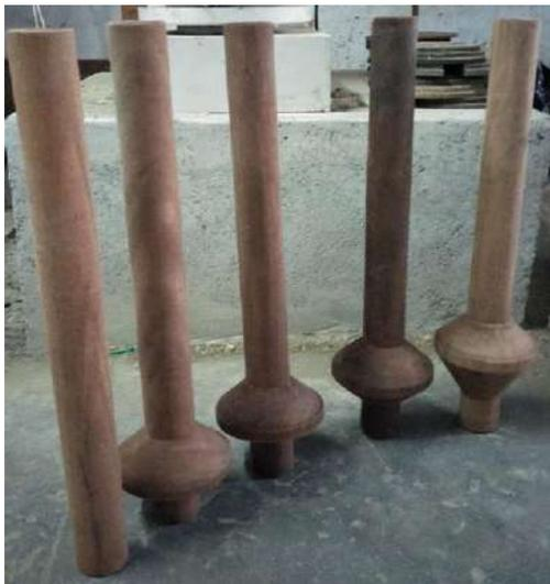
**Fig. 1.** Models of normal and single under-reamed piles.
